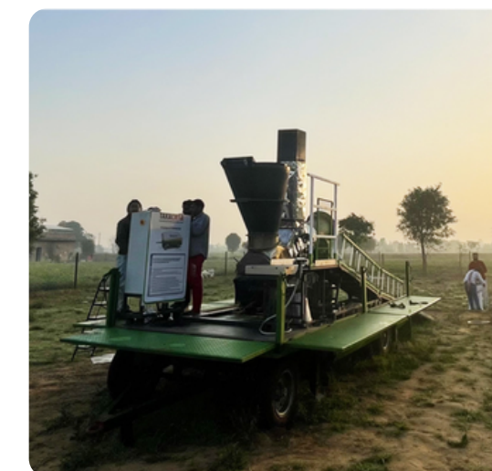
A Takachar Mobile Pyrolysis Unit
