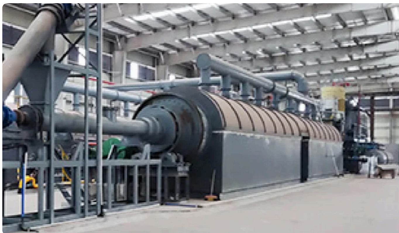
A Continuous Pyrolysis Reactor Image Credit: IndiaMart
